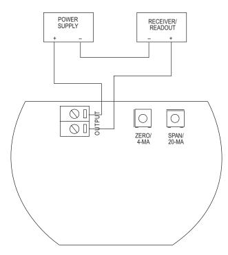
Figure 3: Electrical Wiring Diagram
